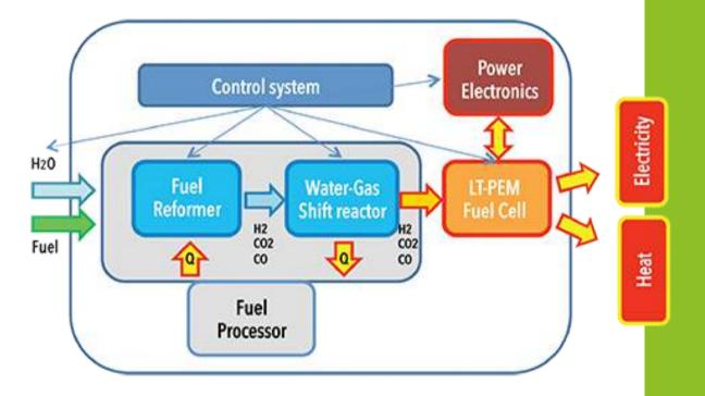
H2PS-5 uses PEM-FCs coupled with a fuel processor based on a reforming step in advance.
