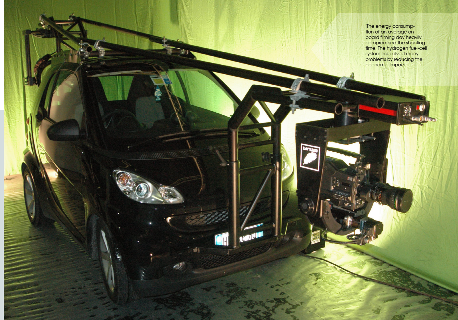
The mechanical arm allows maximum flexibility in film shooting on the move
